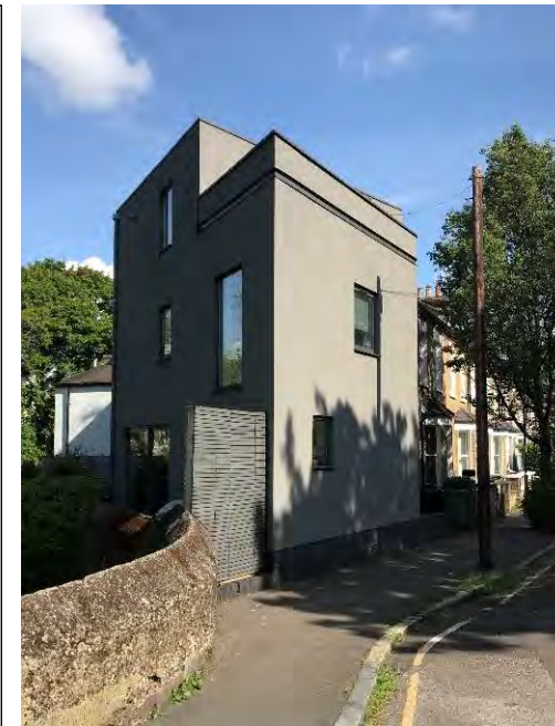
Right. Weardale Road, Lee Forum area. New build house's sharp geometry, accentuated by contrasting render to the adjacent Victorian terrace, is defined by challenging constraints of the infill site, with its riverside location. Fenestration is limited and playful. Setting point lines with frontage of adjacent terrace, and a relief line in the render with adjacent eaves. Top floor is set back to reduce its impact on the street scene. 31/44 Architects
